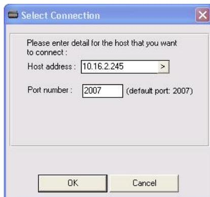
3. Enter in the **Host Address** the IP Address of the SIM Server (The default IP address is 10.16.2.245).
